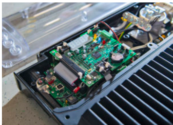
Detail of the electronic board implemented by Elemaster Group mounted on BMS (battery management system) for electric vehicles. (Courtesy of Giuseppe Valentino)
